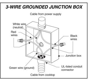
(white) wire is prohibited, you must use a 4-wire power supply cable. Failure to heed this warning may result in electrocution or other serious personal injury.
